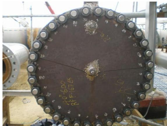
Bolting – During the pressure test the components may be pushed to its limits (almost to yield), it is therefore important the bolting is of adequate strength, the correct grade and that all bolts are fitted (none are missing). There are correct tightening techniques for a bolt ring, to ensure torque is evenly distributed between the individual bolts. Bolts used repeatedly for test purposes should be replaced at regular intervals.
