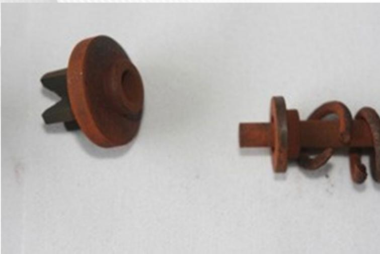
Broken spring, missing ball bearing between seat and spindle
