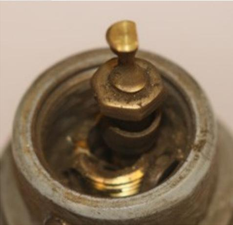
Excessive wear of upper valve guide and damage to valve spindle.
