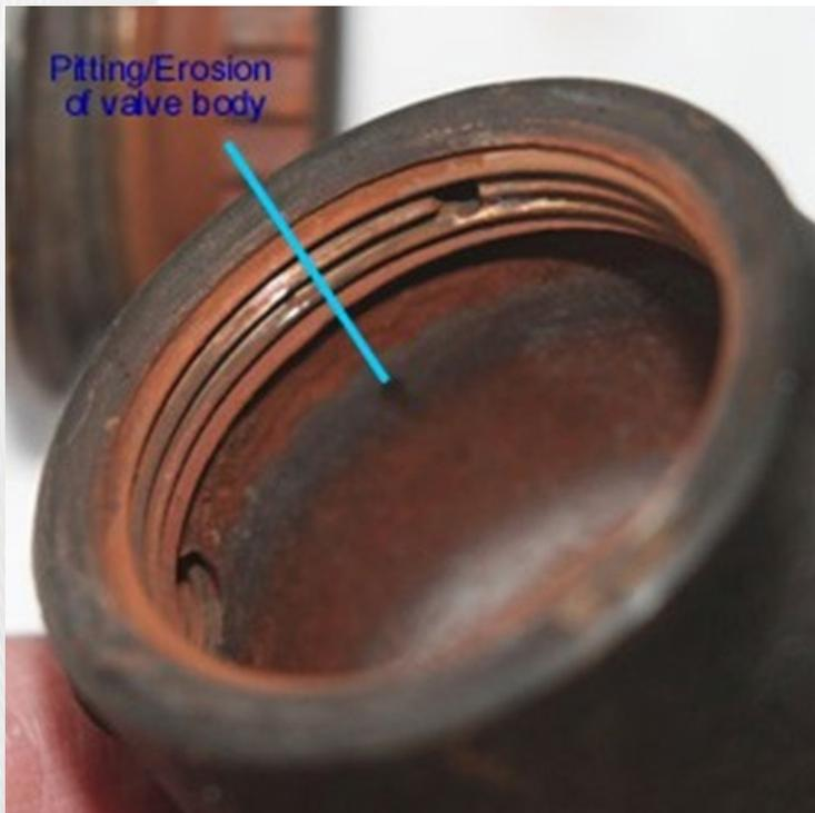
Pitting/corrosion damage on valve body.
