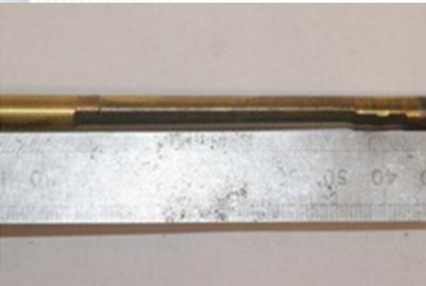
Excessive wear of valve spindle.
