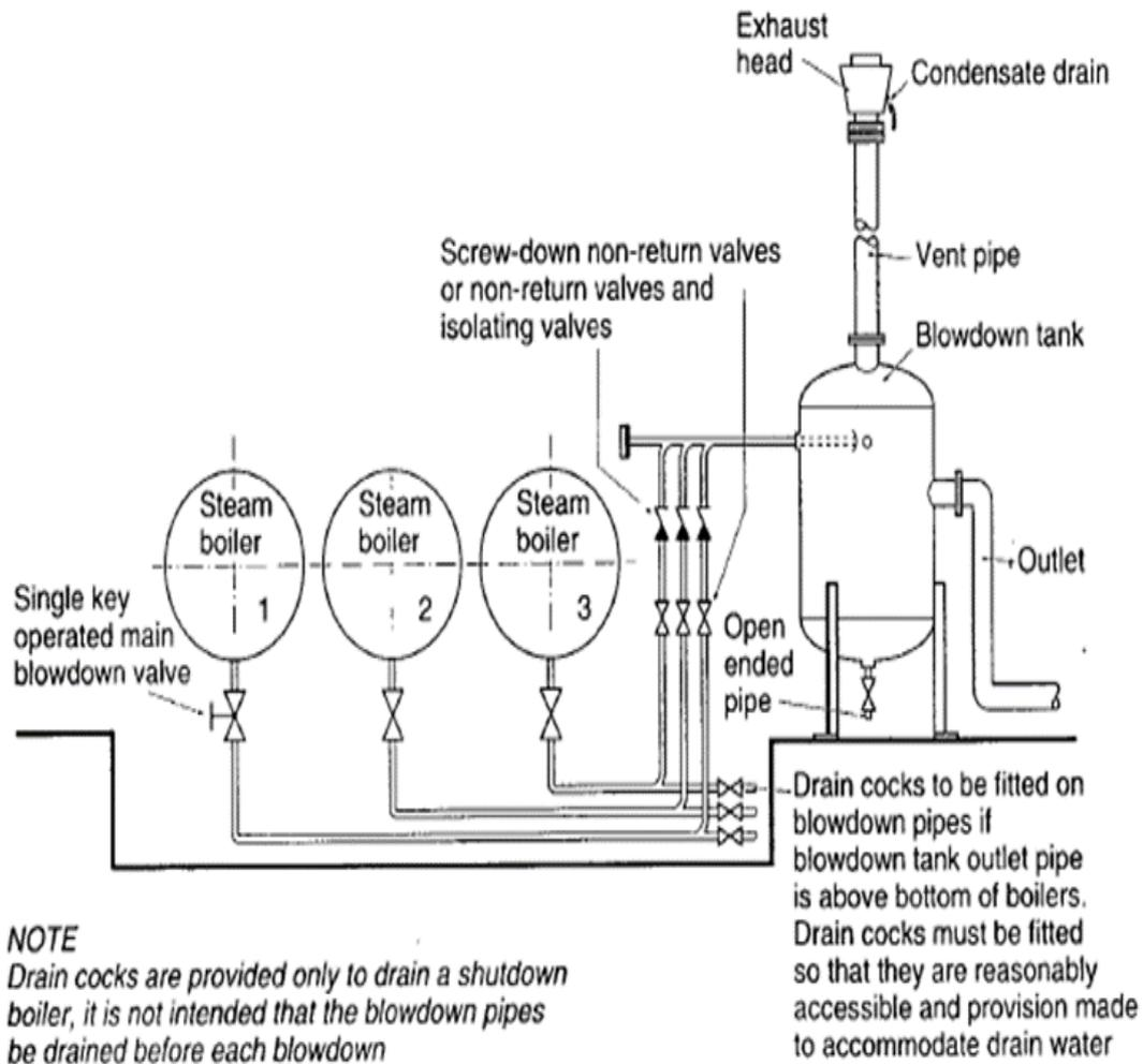
Figure 3 An example of a multiple steam boiler and blowdown tank installation (separate lines from external water level controls and gauge glasses are not shown)
