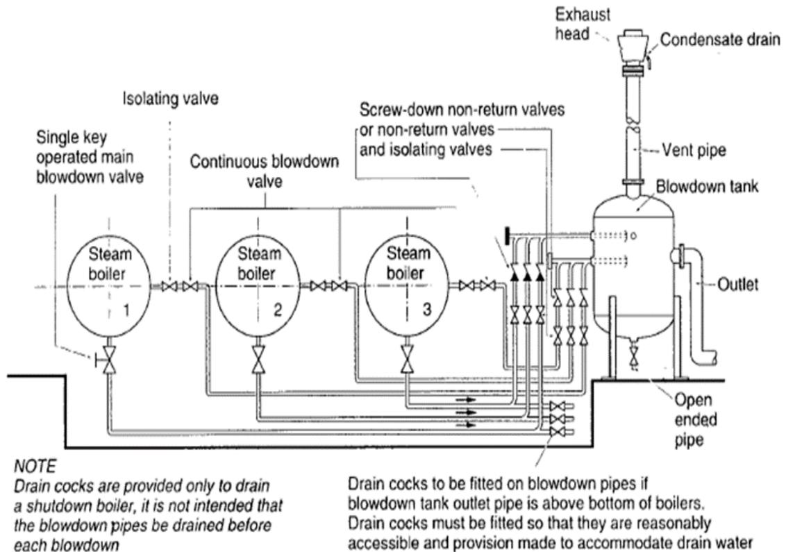
Figure 4 An example of a multiple steam boiler and blowdown tank installation with continuous blowdown (separate lines from external water level controls and gauge glasses are not shown)
