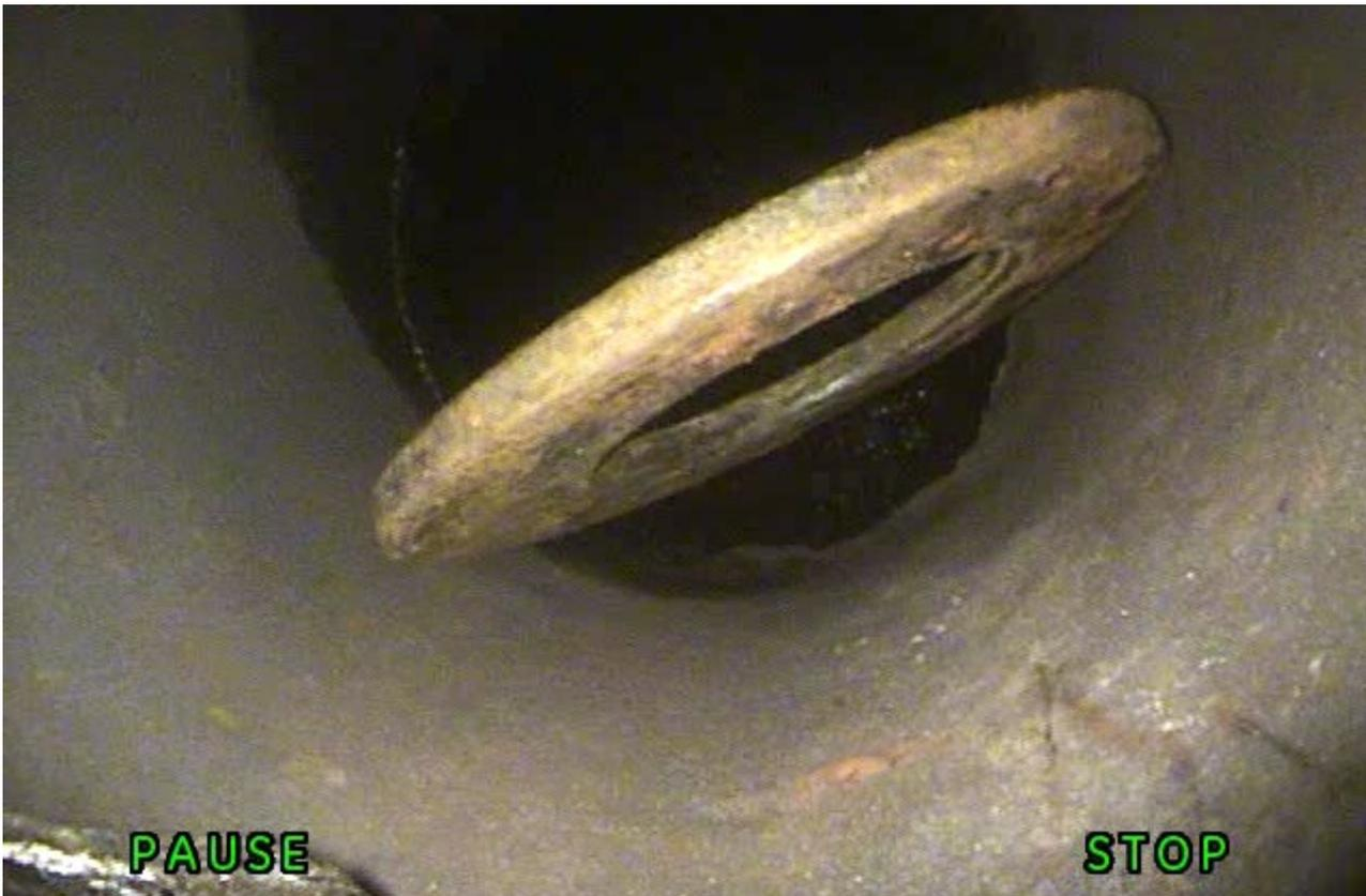
Washer found using articulating borescope in boiler relief line inlet after failure of accumulation test.
