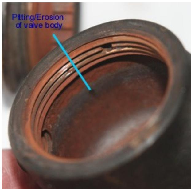
Pitting/corrosion damage on valve body.
