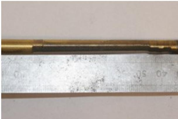
Excessive wear of valve spindle.
