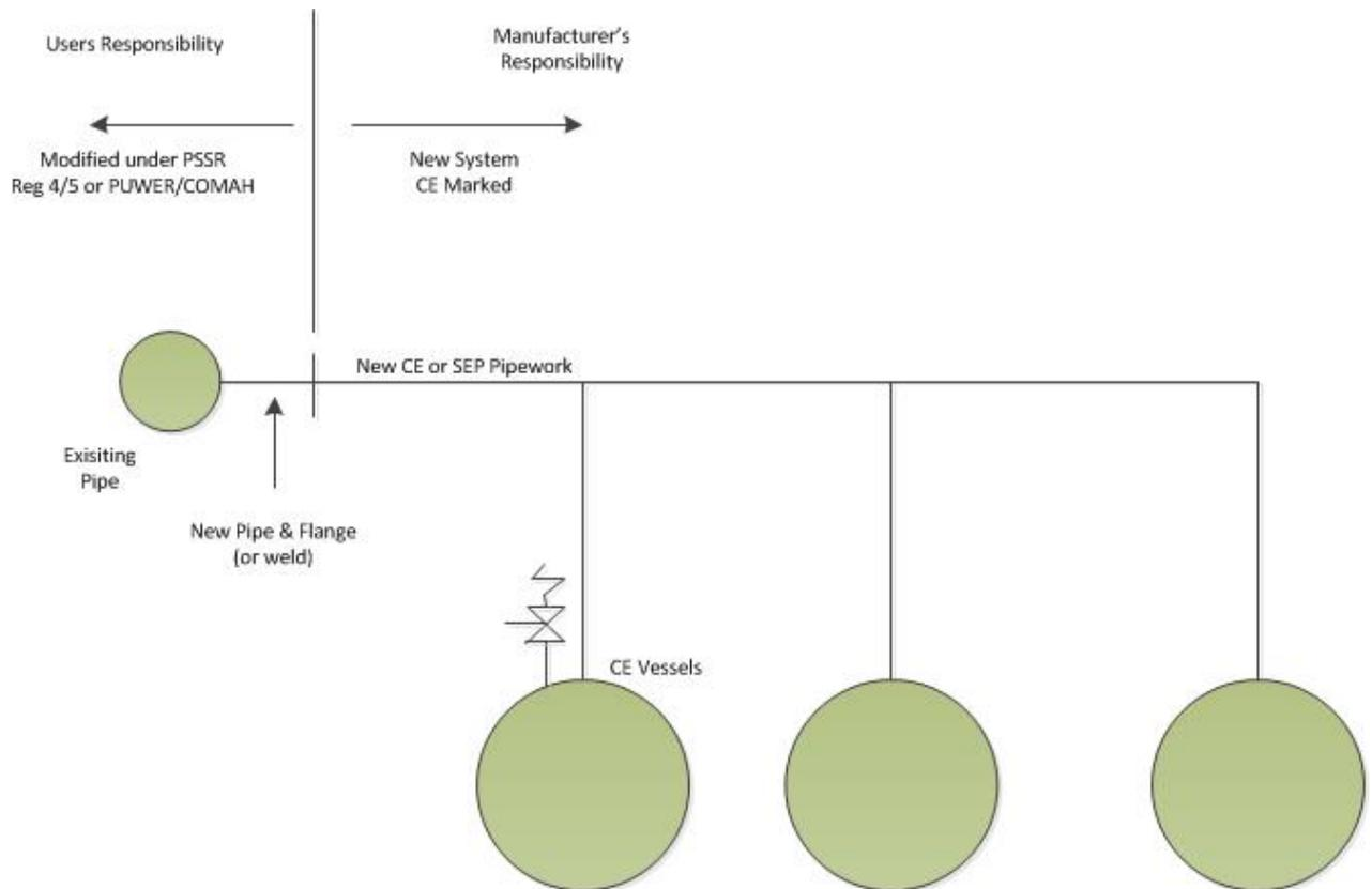
**Fig 3 – How a new assembly should be treated when being added as an extension to an existing installation**
