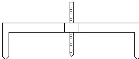
Whether the measurement is to be made internally or externally, the principle is simply to hold the gauge at right angles and perpendicular to the seam with the legs of the gauge in contact with the plate on either side of the seam. The graduated rule is then adjusted until the point is in contact with the shell at the edge of the seam (taking care to avoid any undercut or weld reinforcement). The measurement should then be repeated on the
