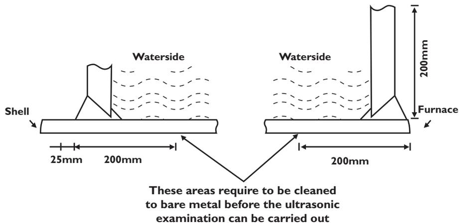
**Figure 2b: NDT preparation areas for set-on end plates**
