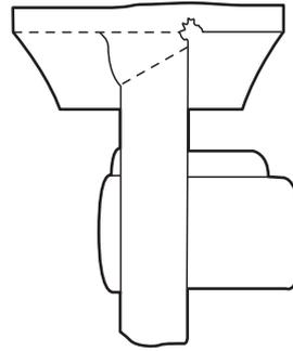
Macrograph of Shell/Endplate and tube connection showing defect propagation in susceptible region
