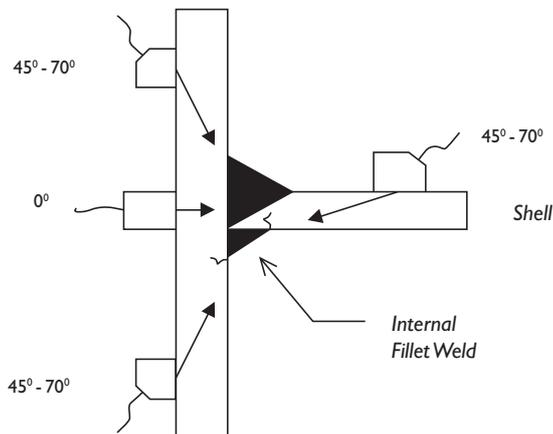
**Note to Figure 2b:** Preparation for Ultrasonic Testing of **set-on** end plates. The endplate and shell surfaces shall be thoroughly cleaned to remove scale for a distance of up to 200 mm back from the toes of the internal fillet weld.
