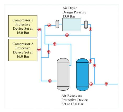
The design and installation failed to consider the maximum pressures of individual components. No consideration was given to global conformity assessment, this showed when the written scheme was created. The design intent was that the air receiver safety valves would protect the dryer, however as air receivers could be bypassed the 13.0 Bar protection for the drier was defeated. Maximum system pressure can be supplied to the dryer.
