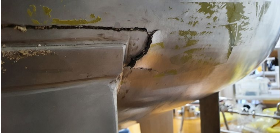
Figure 4. Cracking in leg attachment welds to outer cowling
