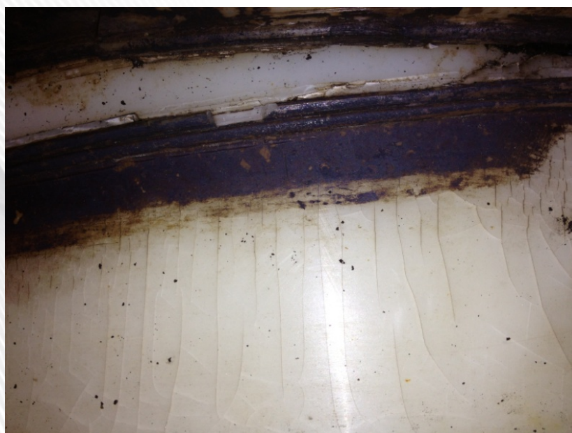
Picture 5 - Degradation due to UV – note the multiple fine cracks
