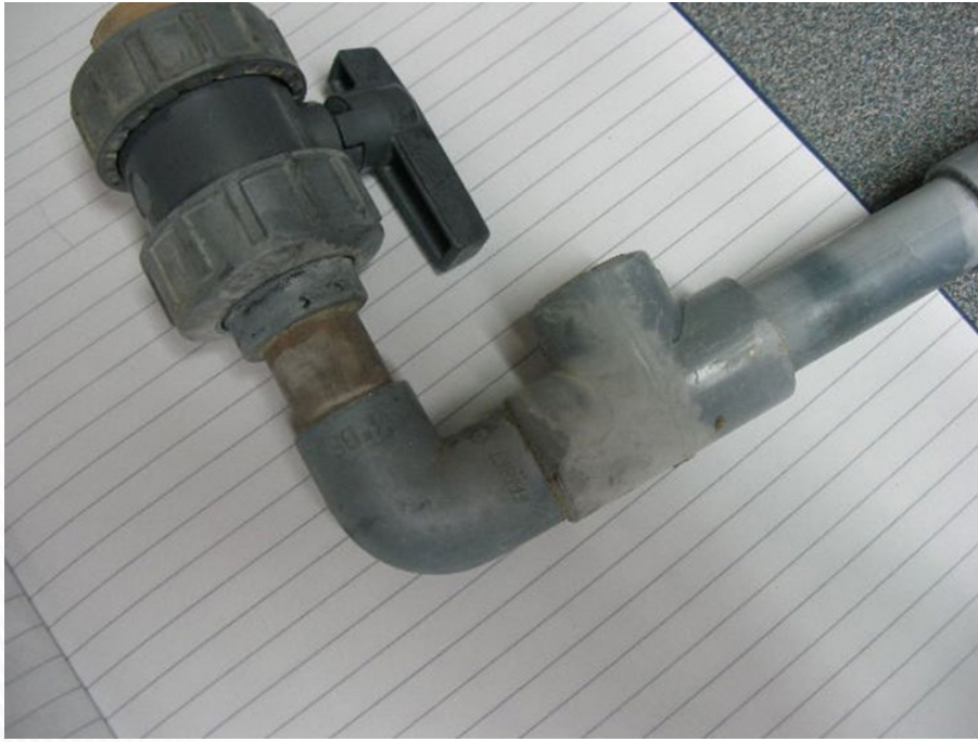
Picture 1- UV degradation – note the change of colour
