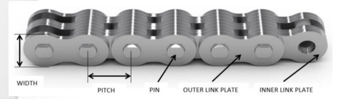
The thorough examination should ascertain the chain plate width as above, is still suitable for further use. Leaf chains which have plate width dimension of less than 95% on the original dimension should be RENEWED PRIOR TO FURTHER USE. The original width can be ascertained at the section of chain near the chain termination which does not travel over pulleys.
