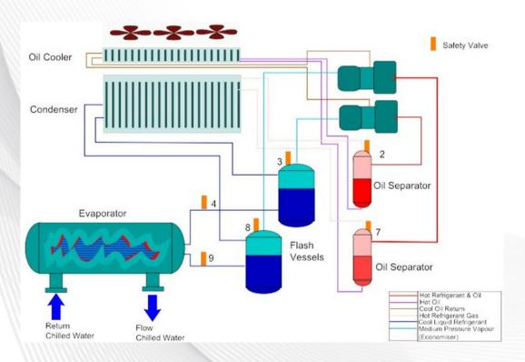
Diagram 1 — Packaged refrigeration system example with a number of typical PE
