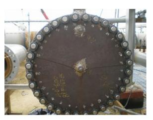
Bolting – During the pressure test the components may be pushed to its limits (almost to yield), it is therefore important the bolting is of adequate strength, the correct grade and that all bolts are fitted (none are missing). There are correct tightening techniques for a bolt ring, to ensure torque is evenly distributed between the individual bolts. Bolts used repeatedly for test purposes should be replaced at regular intervals.
