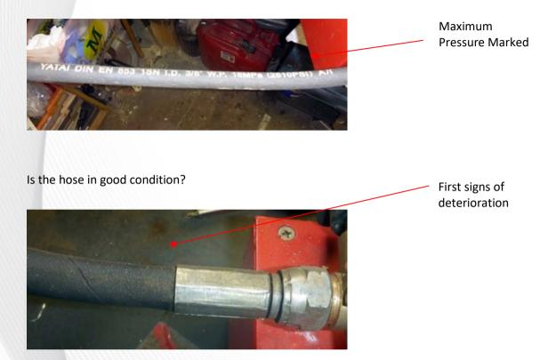
If necessary, test the pump and hose before connection to the component(s).
